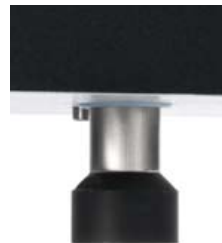
The 5 hammer heads on the underside hit the floor in succession, generating impact sounds.
