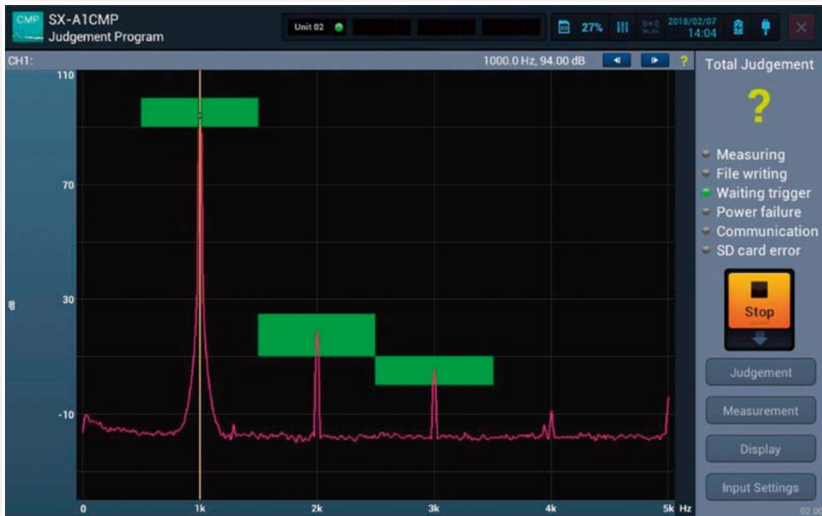
1-channel evaluation screen (Peak evaluation on each frequency domain)
