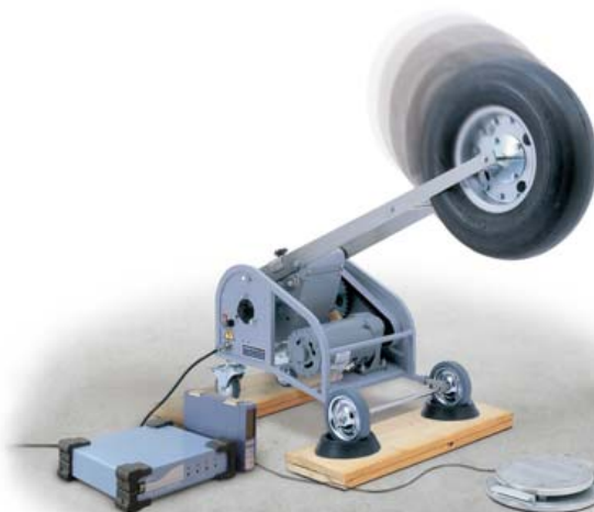
● Example of bang machine impact force measurement
