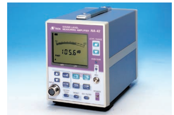
NA-42 sound pressure level measuring amplifier used in the vehicle
