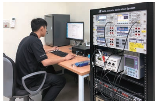
The sound calibration system delivered
