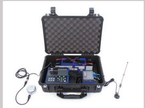
a Live to Web system based upon the Rion XV-2P vibration meter
