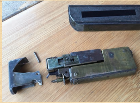
The disassembled parts of a lighter (The ignition unit is shown in the center.)
