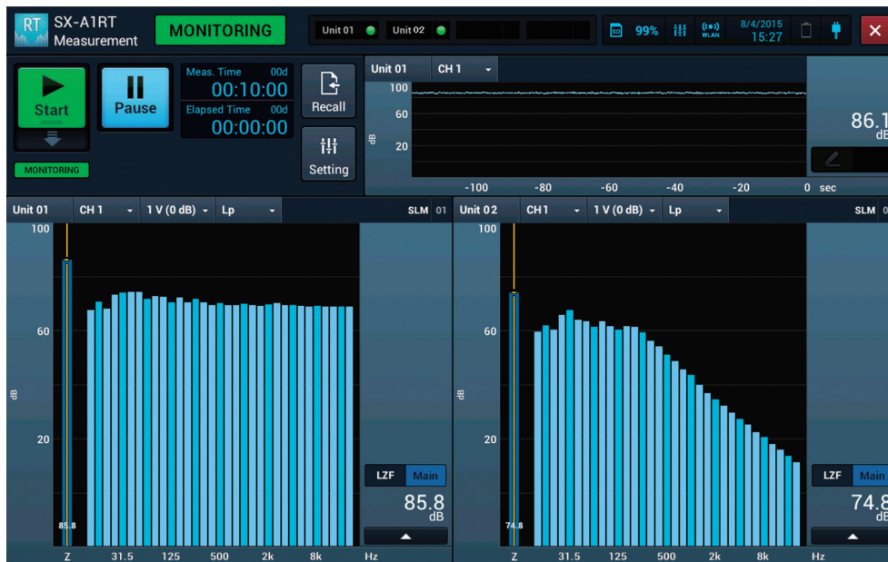
Example for measurement screen of sound pressure level difference between rooms
