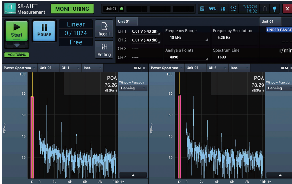
Sample screen for noise FFT analysis and rpm measurement
