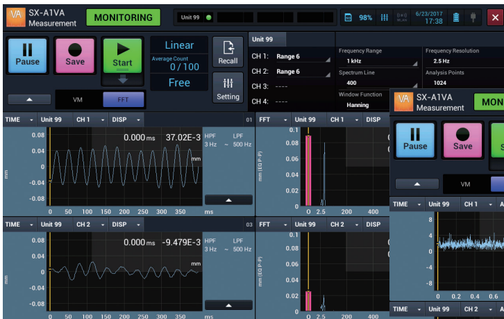
FFT mode 2-channel display (Unbalanced condition)
