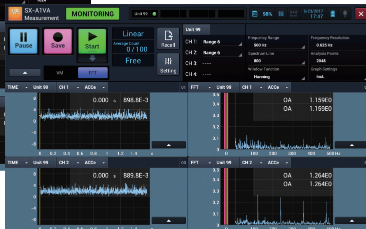
FFT mode 2-channel display (bearing problem)
