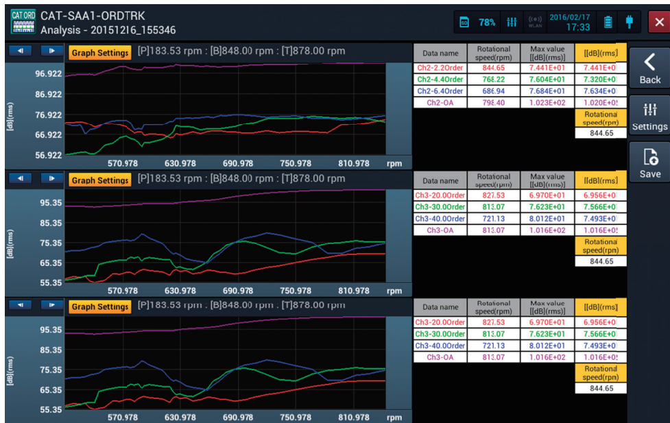
RPM - Level (Simultaneous display of multiple orders)
