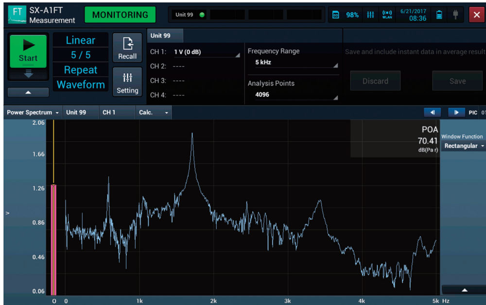
Screen example for FFT analysis of impact sound
