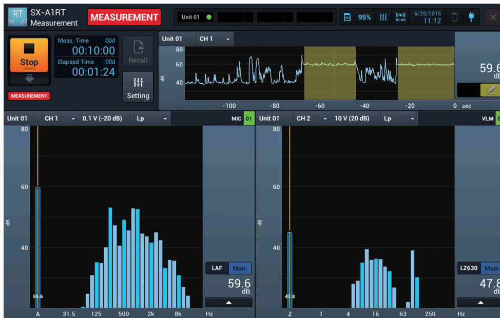
Example of multi-channel octave band analysis and real-time analysis (using the auto store function of SX-A1RT)
