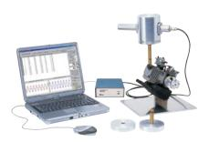
Regardless of the shape, the combustion chamber volume can be measured by simply placing the volume meter on the combustion chamber cavity of the cylinder head, as shown in the picture.
