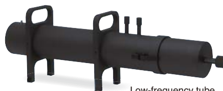
Low-frequency tube (internal diameter 100 mm)
