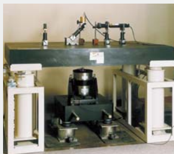
Absolute calibration setup for vibration accelerometers
